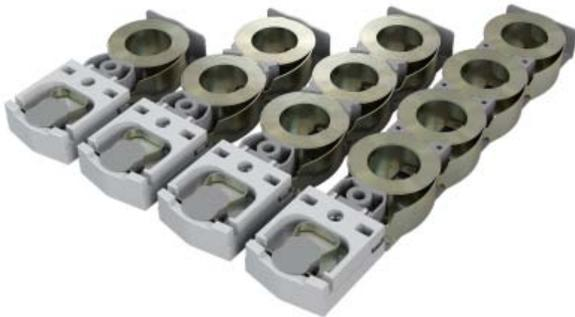
The 984 series is a standard mount constant force system. The interlocking coils give the customer a modular solution to achieve the exact coil weight to match the sash weight. Mounted below the tilt latch, it gives good protection to dirt and debris in new construction environments.
